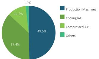
A detailed analysis of how consumption is distributed at our plants shows that production machinery, cooling and air conditioning units consume roughly 86% of the electric energy. Compressed air production is another significant energy driver. These are the two areas that our teams are focusing on. Together with consultants they are developing concepts to improve our performance, either by investments in more modern facilities or by increasing efficiency.
