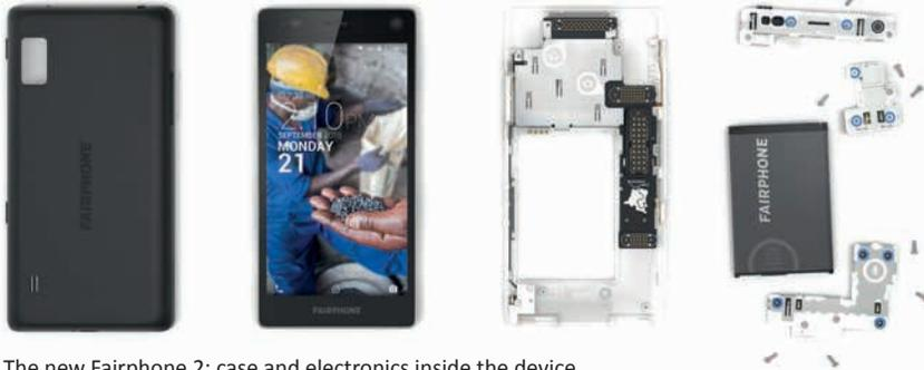
The new Fairphone 2: case and electronics inside the device
