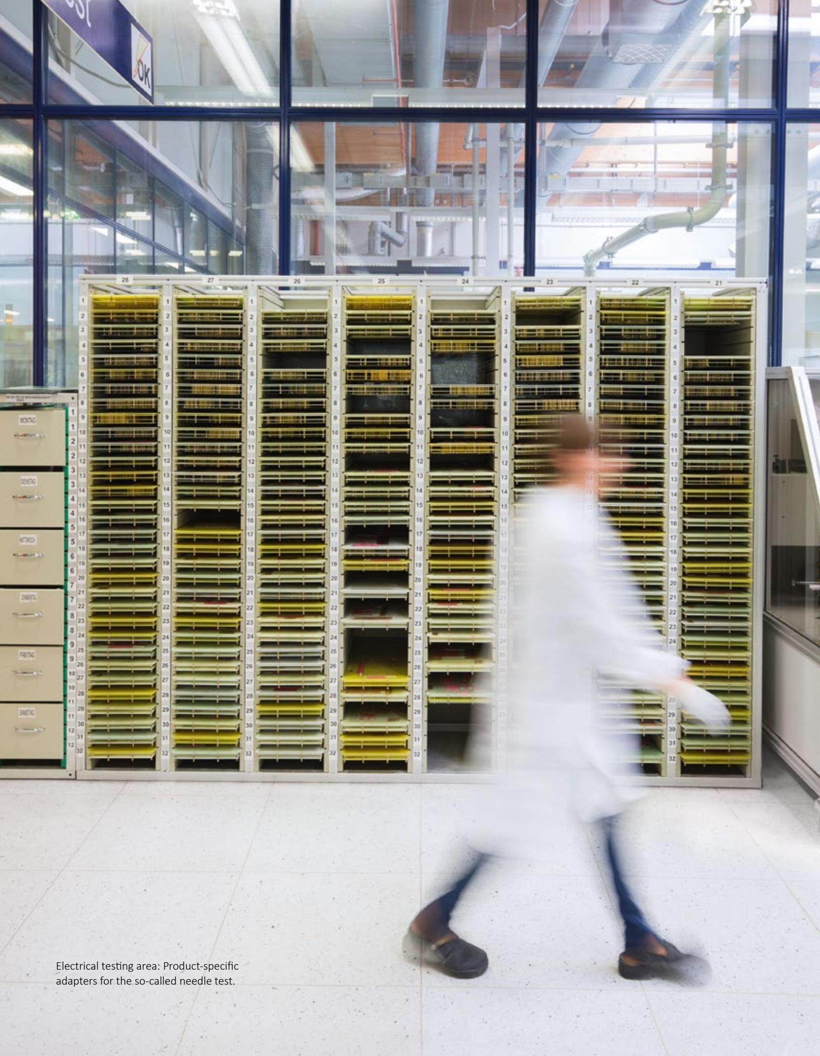
Electrical testing area: Product-specific adapters for the so-called needle test.
