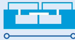
Embedded and surface-mounted components (reduced footprint, shorter connection)
