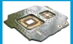
This technology platform combines mechanical and electronic miniaturisation. It enables partial reduction of the thickness of a circuit board, so that populated assemblies have a thinner profile. Additionally, it can be used to make cavities in the printed circuit board, for example for acoustic channels. A major application for this technology is the 2.5D® rigid-flex printed circuit board, a lower cost alternative for flex-to-install applications.
