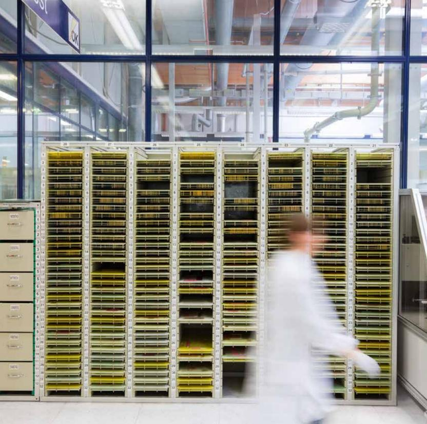
Electrical testing area: Product-specific adapters for the so called "needle test".
